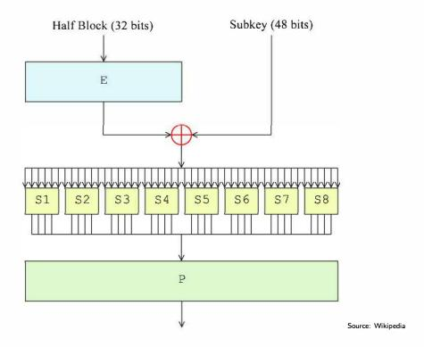
It takes as input a half-block (32 bits) and a subkey (48 bits), and produces 32 bits of output.
