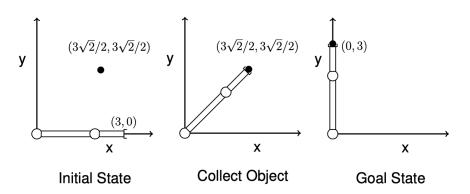
The goal of the robot is to collect an object placed at coordinates  $(3\sqrt{2}/2, 3\sqrt{2}/2)$  and move this object to the position identified by coordinates (0, 3), as shown in the Collect Object and Goal State figure above, respectively. This problem can be formulated as a search problem as follows:
